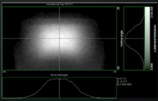
The flood light provides a low, wide angle light pattern to increase short-range visibility. Ideal for added safety in fog, sleet and rain
